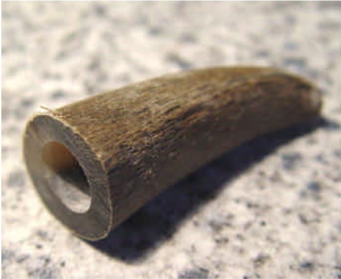
**At the following steps great attention has to be paid to the accuracy of the cone. If one bores an uneven (non circular) cone one has a genuine problem, because the depression can be filled up with epoxy and be sanded but you might see this later –depending on how this the horn becomes here- in front of the bright wood.**
