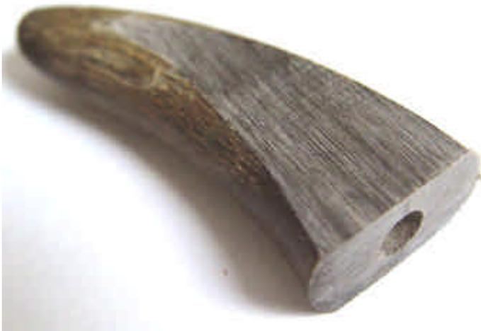
Subsequently, pre-drilled with 3mm first and counerbored with 6,5mm and finally conically bored with a cone skaped rasp (6,5mm being the smaller cone dimeter on my bow end). The stench is bearable if one holds back oneself with the number of revolutions. If the horn becomes too hot and burns it will also bake to the drill and is quite hard to get it off the tool > file brush)
