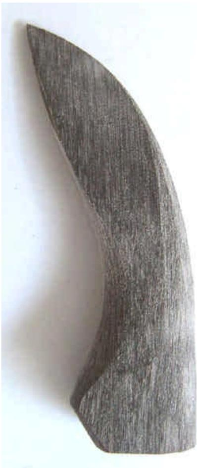
With this step one must watch out much that one does not sand the lower –open- edge too thin. At my nock it was still about 1mm.
